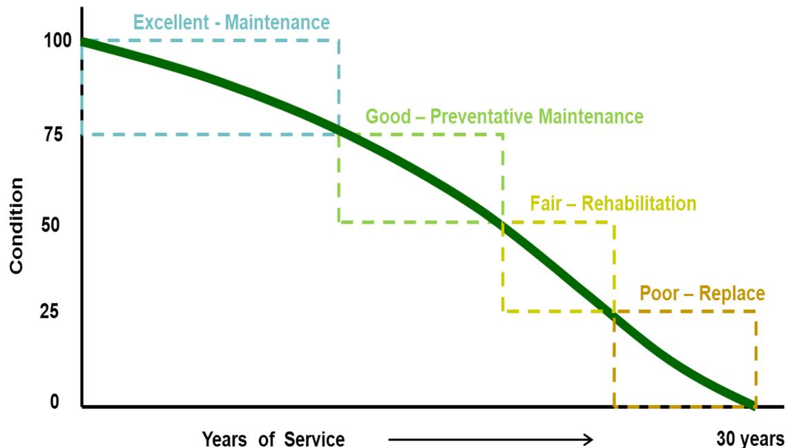
As shown above, during the road's life cycle there are various windows available for work activity that will maintain or extend the life of the asset. These windows are: maintenance; preventative maintenance; rehabilitation; and replacement or reconstruction.
