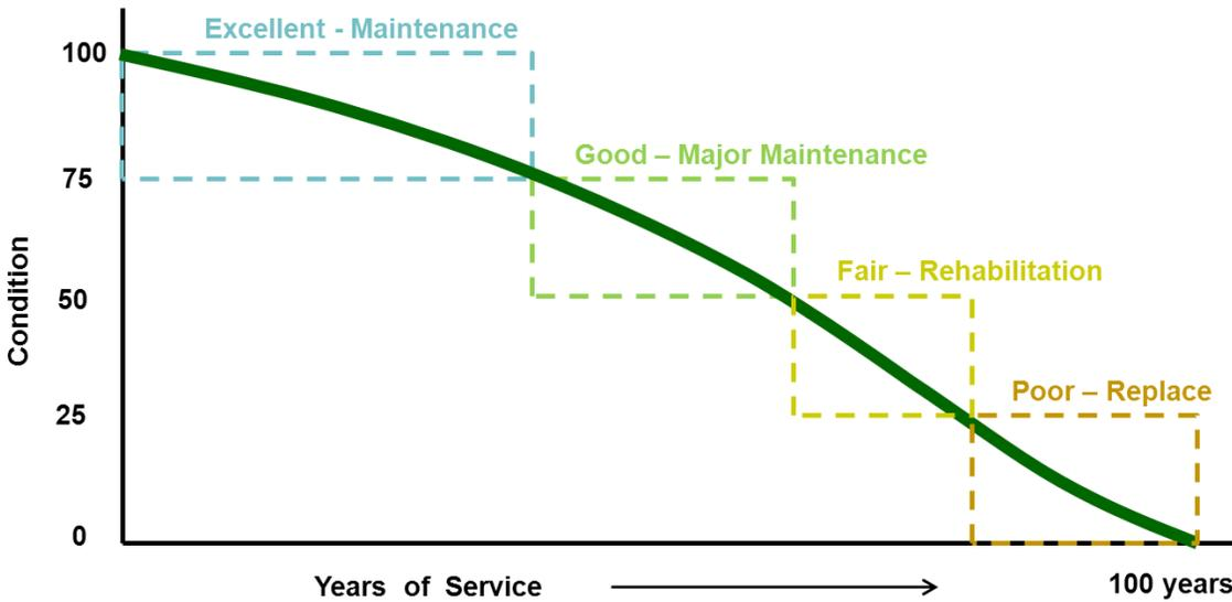
As shown above, during the sewer main’s life cycle there are various windows available for work activity that will maintain or extend the life of the asset. These windows are: maintenance; major maintenance; rehabilitation; and replacement or reconstruction.
