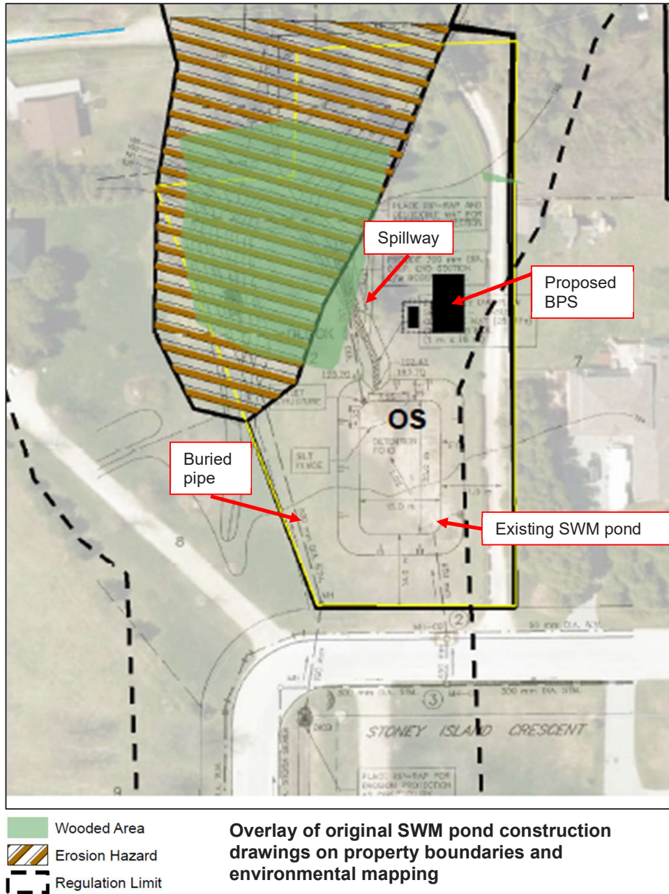
Figure 11: Conceptual Revised Location of a BPS located on the SWM Pond site (as presented at PIC2)
